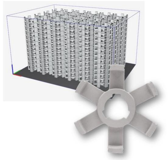
This stator is designed for use in a small electric motor.
